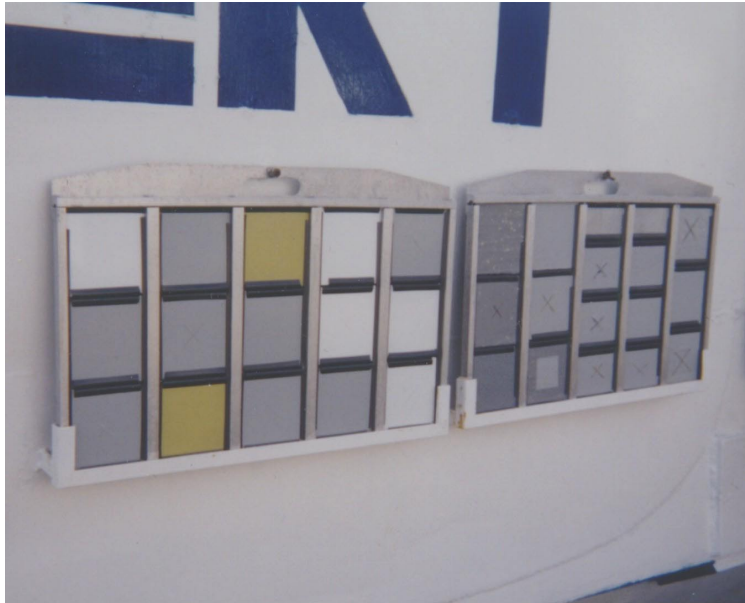
Figure 6. Left: Test panels mounted on ship. Right: Sensor measurements showing degradation of a coating exposed on a ship in Hawaii.
