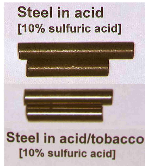
Figure 7. Attack on steel by 10% sulfuric acid with and without tobacco extract. Left: weight loss; right: steel rods after immersion.
