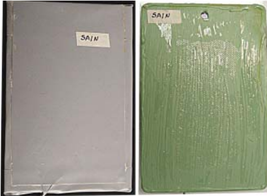
Example of steel specimens after salt fog exposure before and after removal of no-defect appliqué.
