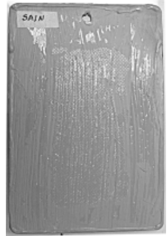
Figure 2. Example of no-defect steel specimens after appliqué removal.
