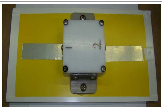
Figure 3. Painted panel with mounted CHM and tape electrodes.
